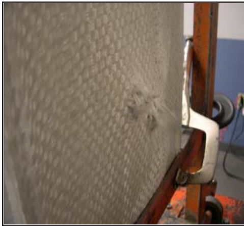
Back Face UL 752 Level III Test Shot
