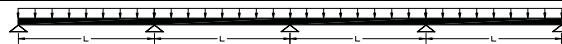
Design Charts for SuperWale™ Specified with Vinyl Ester Resin -Simply Supported, Continuous Span Load Condition, Metric Units
