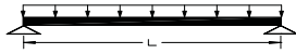
Design Charts for SuperWale™ Specified with Vinyl Ester Resin -Simply Supported, Simple Span Load Condition, Imperial Units
