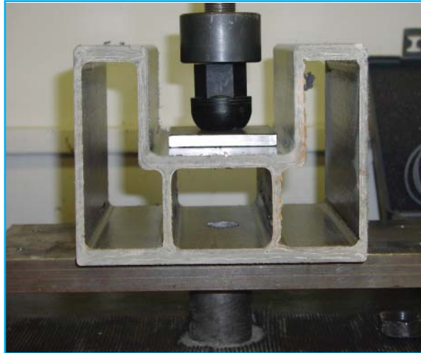
Figure 1. Photo of the Tie-rod push through test conducted in CPI Lab.
